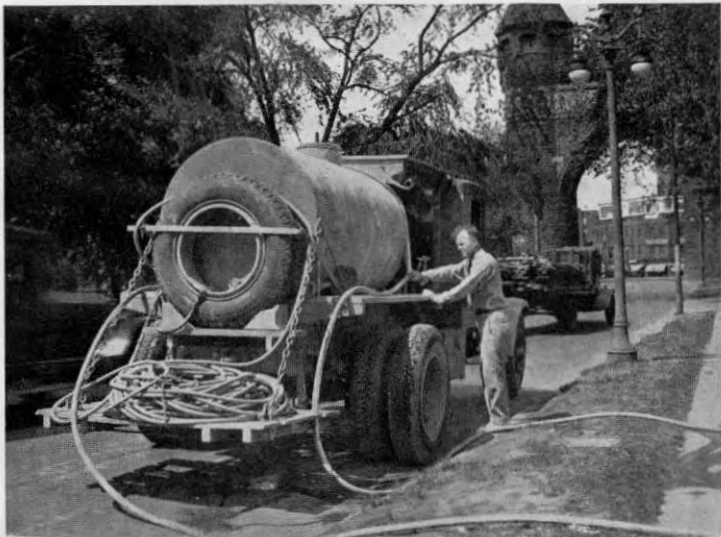
b. View of power sprayer outfit used in treating lawns with lead arsenate.
