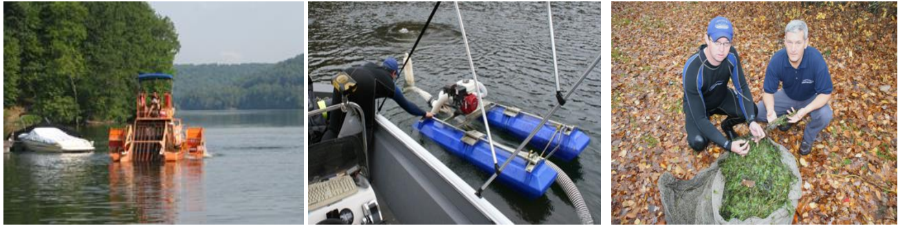
Figure 11. Mechanical harvester (left), suction harvester (middle), plants from suction harvesting (right).
