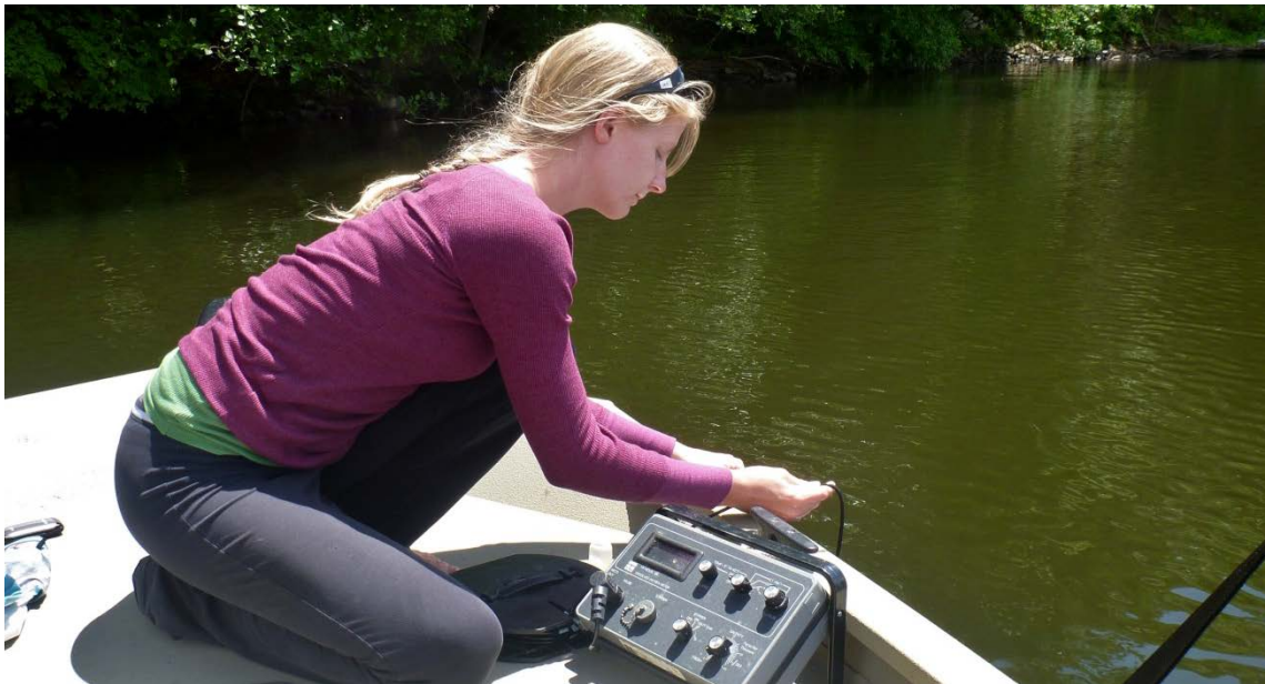
Figure 2. Testing water for temperature and dissolved oxygen in Lake Zoar.
