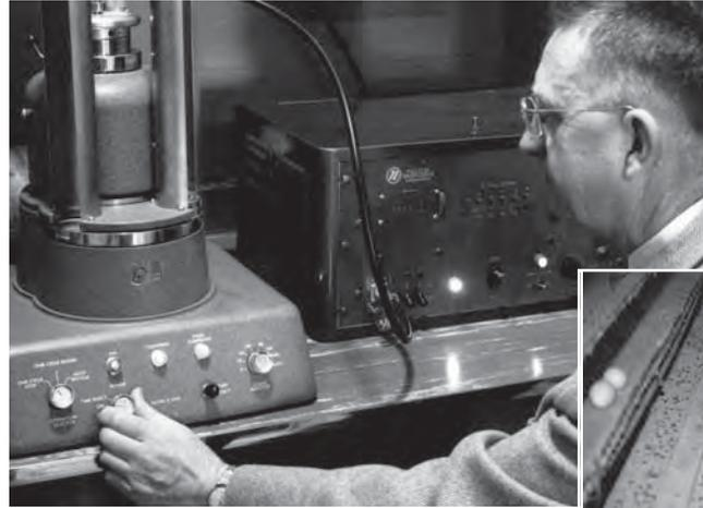
Figure 43. Dr. Raimon L. Beard, using a Thin-Window Counter (early radiation detector), 1961.
